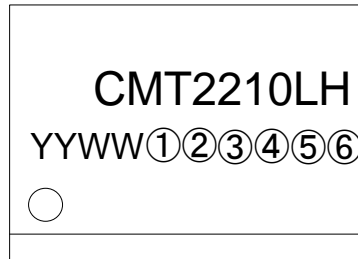
Figure 12. CMT2210LH Top Marking
