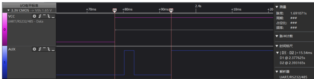
Figure 4 Power-on startup timing diagram
