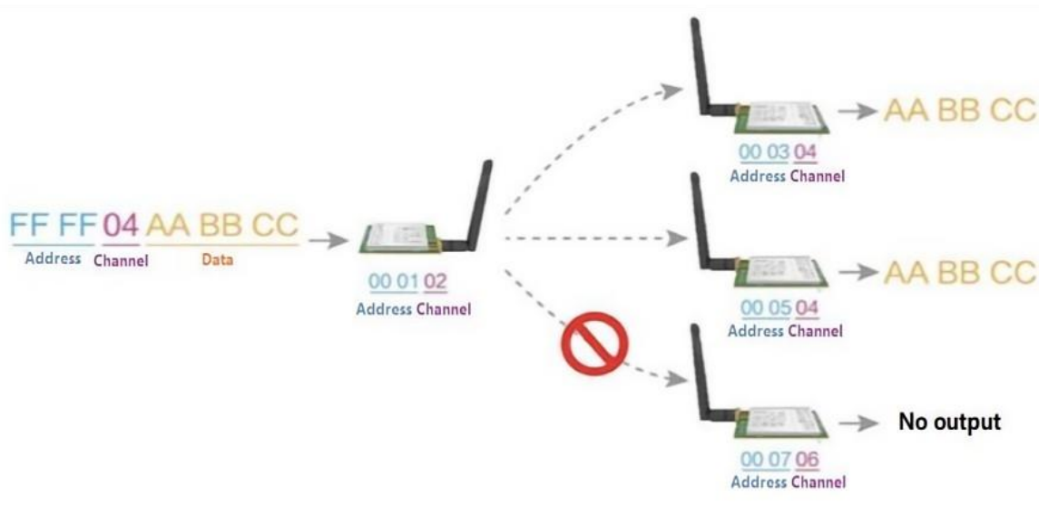
Fig. 2 Schematic diagram of fixed-point broadcast transmission
