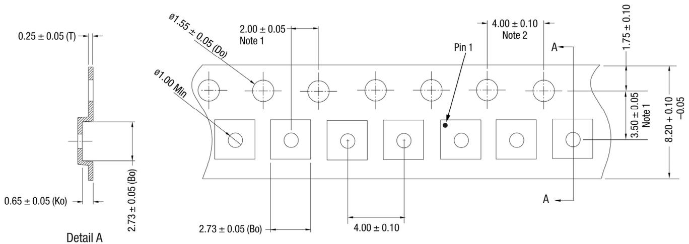
**Figure 6. RFX8422S Tape and Reel Dimensions**
